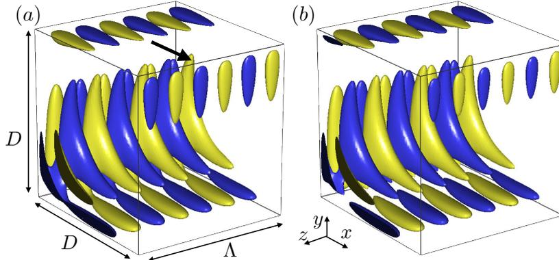
FIGURE 1. Representation of TGL vortices in the lid-driven cavity flow at  $Re = 1200$  and  $\Lambda/D = 0.945$ ; lid moves in the direction of arrow. Snapshot of iso-surfaces of 20% max/min spanwise velocity of spanwise Fourier mode  $\beta = 3$ . (a) DNS, (b) resolvent-based model. Animations of iso-surfaces of DNS and model are shown in supplementary movies 1 and 2 respectively.
