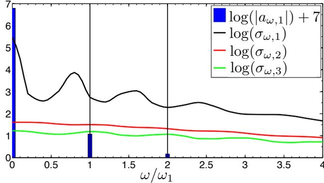
FIGURE 3. Bars correspond to the (scaled) amplitude of the resolvent modes associated to each frequency at  $\beta = 3$ . Lines denote the distribution in frequency of the first, second and third singular value at  $\beta = 3$ .
