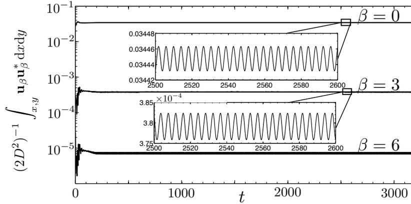
FIGURE 2. Temporal evolution of the kinetic energy based on (2.2) of the three most energetic spanwise Fourier modes. Mode  $\beta = 0$  contains the mean flow while  $\beta = 3$  consist of three pairs of TGL vortices. Self-interaction of mode  $\beta = 3$  provides energy to its harmonic  $\beta = 6$ .
