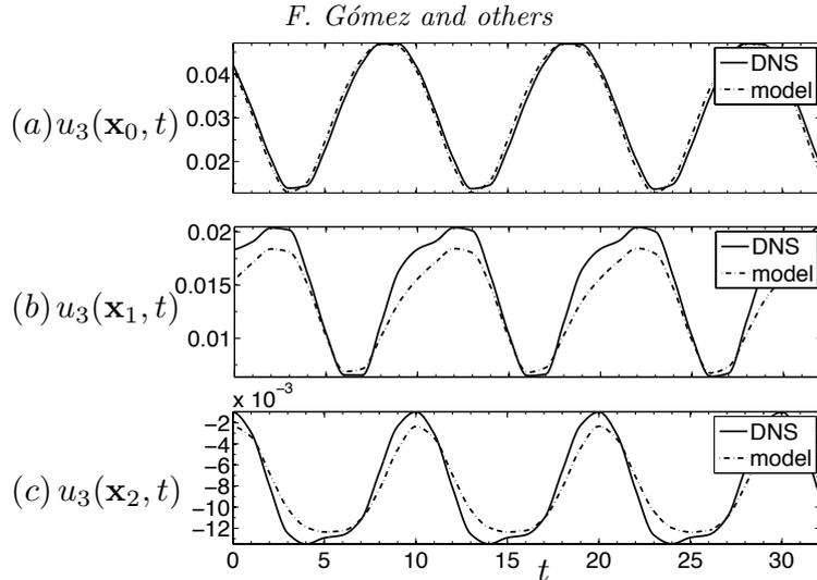
FIGURE 5. (a) Temporal evolution of the real part of the velocity component  $u$  at the location  $\mathbf{x}_0 = (0.1, 0.1, 0)$  at  $\beta = 3$  obtained via DNS. The dashed line indicate the temporal evolution of the resolvent-based model at  $\mathbf{x}_0$  with probe location at same point. (b) DNS and model signals at  $\mathbf{x}_1 = (0.82, 0.95)$  with probe location at  $\mathbf{x}_0$  (c) DNS and model signals at  $\mathbf{x}_2 = (0.4, 0.26)$  with probe location at  $\mathbf{x}_0$ .
